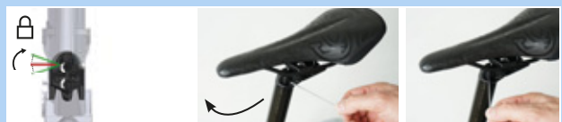
Figure 184: Closing the height adjustment
