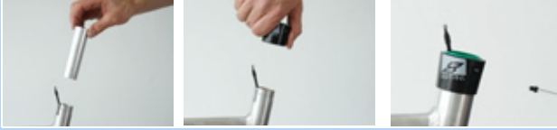
Figure 204: Fitting the slide bushing and outer sleeve
