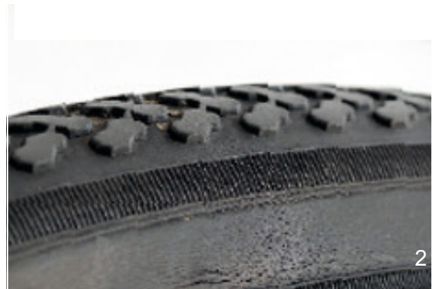
Figure 135: Examples of fatigue cracks (1) and ageing cracks (2)
