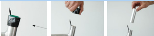
Figure 155: Removing the outer sleeve and slide bushing
