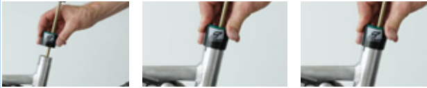
Figure 179: Attaching the outer sleeve
