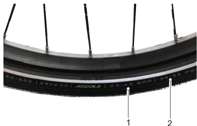
Figure 133: Tyre pressure in bar (1) and psi (2)
