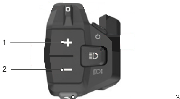
Figure 121: Position of plus (1), minus (2), and push assist (3) buttons
